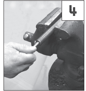
4. Insert splice core into cable one turn.
